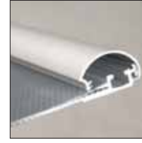
Profile / UYUP003400 26 mm Aluminium Snap profile set (top & bottom) in 3 meters without springs. Top Profile is silver anodized. Bottom profile is mill finished.
